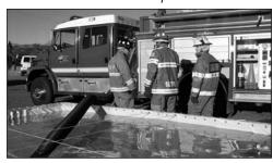
An engine drafts water from a 3000-gallon portable tank during a drill.
